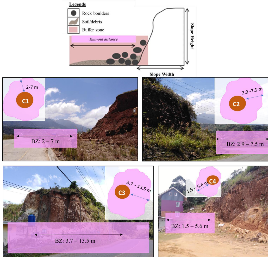
Figure 6. (Above) Sketch of buffer zone estimation based on run-out distance, (Below) Buffer zone estimation for research slopes in the research area
