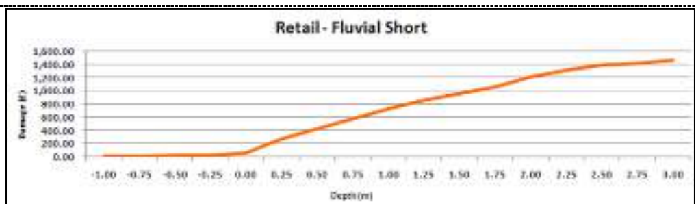
Figure 2. Example Flood Stage-Damage Curve for retail building in MCM Handbook (Penning-Roswell et.al., 2013)
