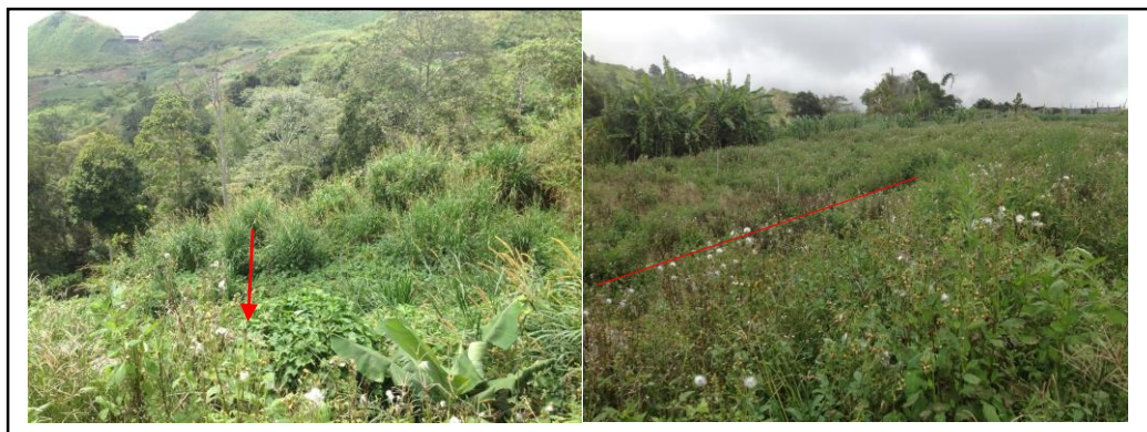
Figure 5. Field verification of a landslide (Figure 3c) indicating straight line of scarp by observing vegetation pattern and sudden drop of plantation area.
