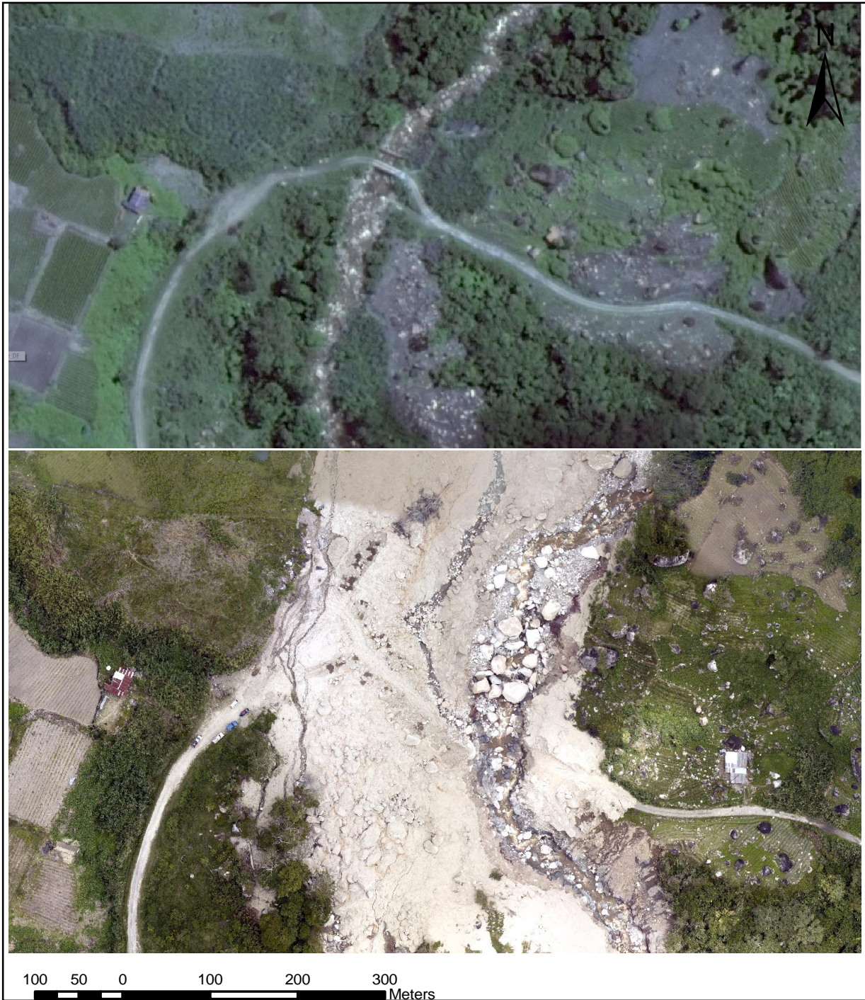
Figure 7. Multi temporal images disconnected roads before debris flow from Worldview image in 2011 (top) and after debris flow from orthophoto in 2015 (below). 5m of road was displaced after the debris flow event.
